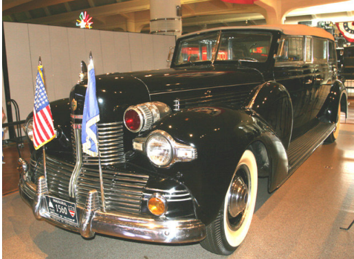
The "Sunshine Special", a 1939 Lincoln K used by Presidents Roosevelt and Harry Truman. On display at the Ford Museum. With amour plating, special windows and other equipment, it weighed in at 9300 pounds
