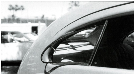
Stylish wind wing in the tear drop rear window was standard equipment.
