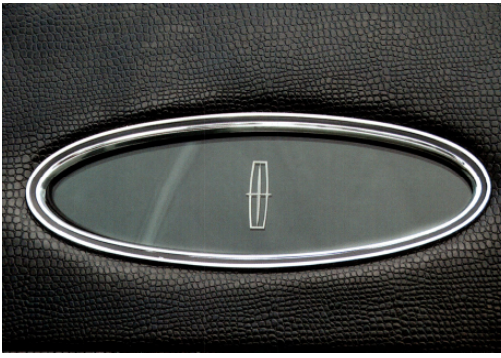
These distinctive oval shaped windows, with the Lincoln star were part of the rear sail panels
