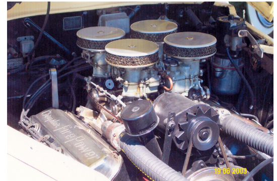
The four carburetors on the Hemi engine in Rod Johnson's 1948 Continental.
