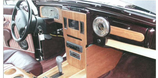
Another view of the custom interior, incorporating instruments and steering wheel from a Mark VIII. Clock is from a 1948 Continental.
