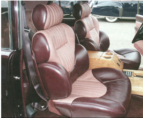
Custom interior features bucket seating from a Pontiac Bonneville. They look and feel great.
