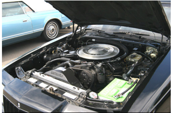
No garden variety MK VII engine here, lurking under the hood is a 351 Windsor block.
