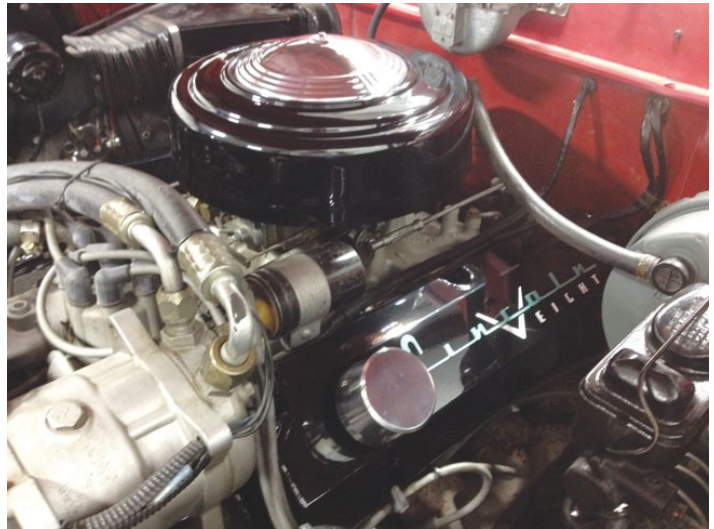
Where the power lives. Not your stock 317 Lincoln V8, this is a Ford 351 cubic inch motor, coupled to a Ford C6 three speed automatic. Note the A/C compressor to the left. This is one very interesting and sweet Lincoln.
