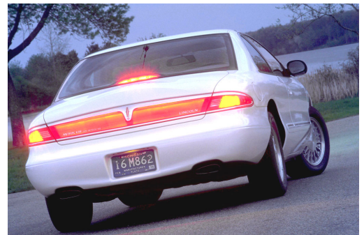
1997 and 1998 Mark VIIIs feature a neon glow system for rear tail lamps.
