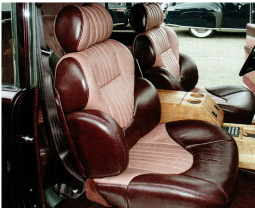
The front seats for this custom Continental are from a Pontiac Bonneville. While not FOMOCO, they still provide comfort to the max for both passenger and driver-and who does really want to be comfortable.
