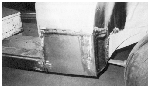
The bottom six inches of the entire body was replaced with new metal due to the severe rust damage.
