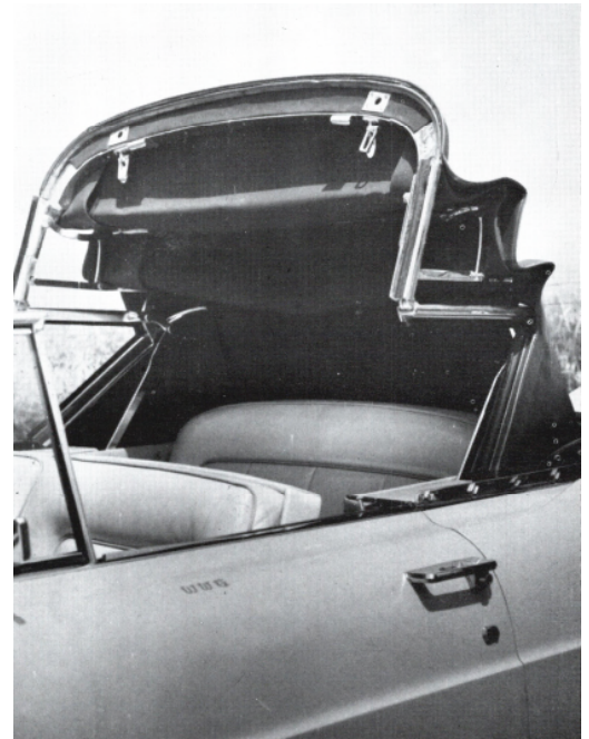
Top mechanism in action on the Mark II. Walter E. Goepfinger had his initials placed near the top of each door.
