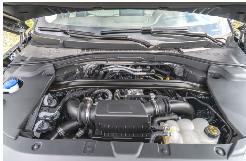
The engine compartment showing the twin-turbocharged V-6 engine, producing 400 horsepower in standard form.
