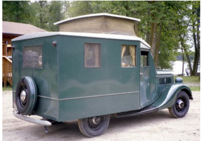
1937 Ford House Car was produced in very limited numbers at the Ford Plant in St. Paul, Minnesota. The body is framed and paneled in wood, with sheet steel cladding.
