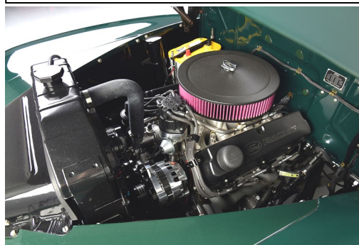
A very modern Ford 302 engine makes for a great running 1947 woody wagon.
