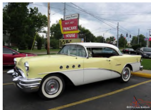
1955 Buick Century two door hardtop, replete with the famous four portholes, signifying the large Roadmaster engine in the small Special body.
